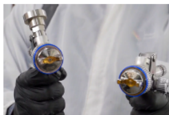
Image depicts two spray paint guns with two different nozzle sizes.
