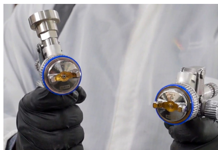
Image depicts two spray paint guns with two different nozzle sizes.
