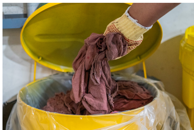
Wear PPE when handling rags, wipes or towels that have been used with solvents, chemicals or oils.
