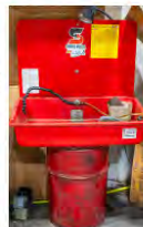
A commonly used drum-mounted parts washer.
