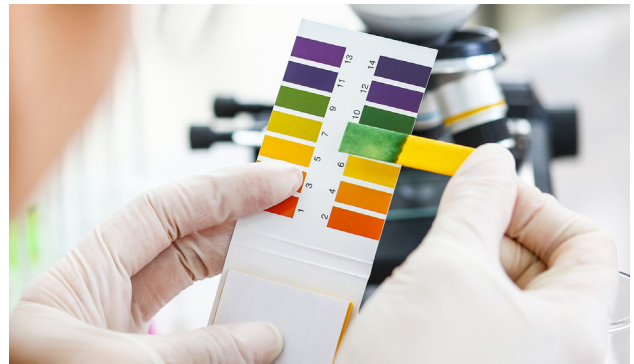
Low-cost pH tests can help monitor water-based cleaning solution effectiveness – acidity vs. alkalinity.
