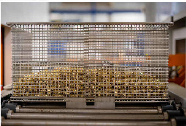
Micro-parts that are draining in a basket after going through a parts washer.
