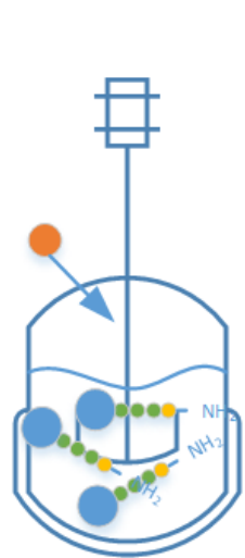
SPPS (linear) Fmoc-AA chemistry >3 eq AA and reagents DMF and NMP
