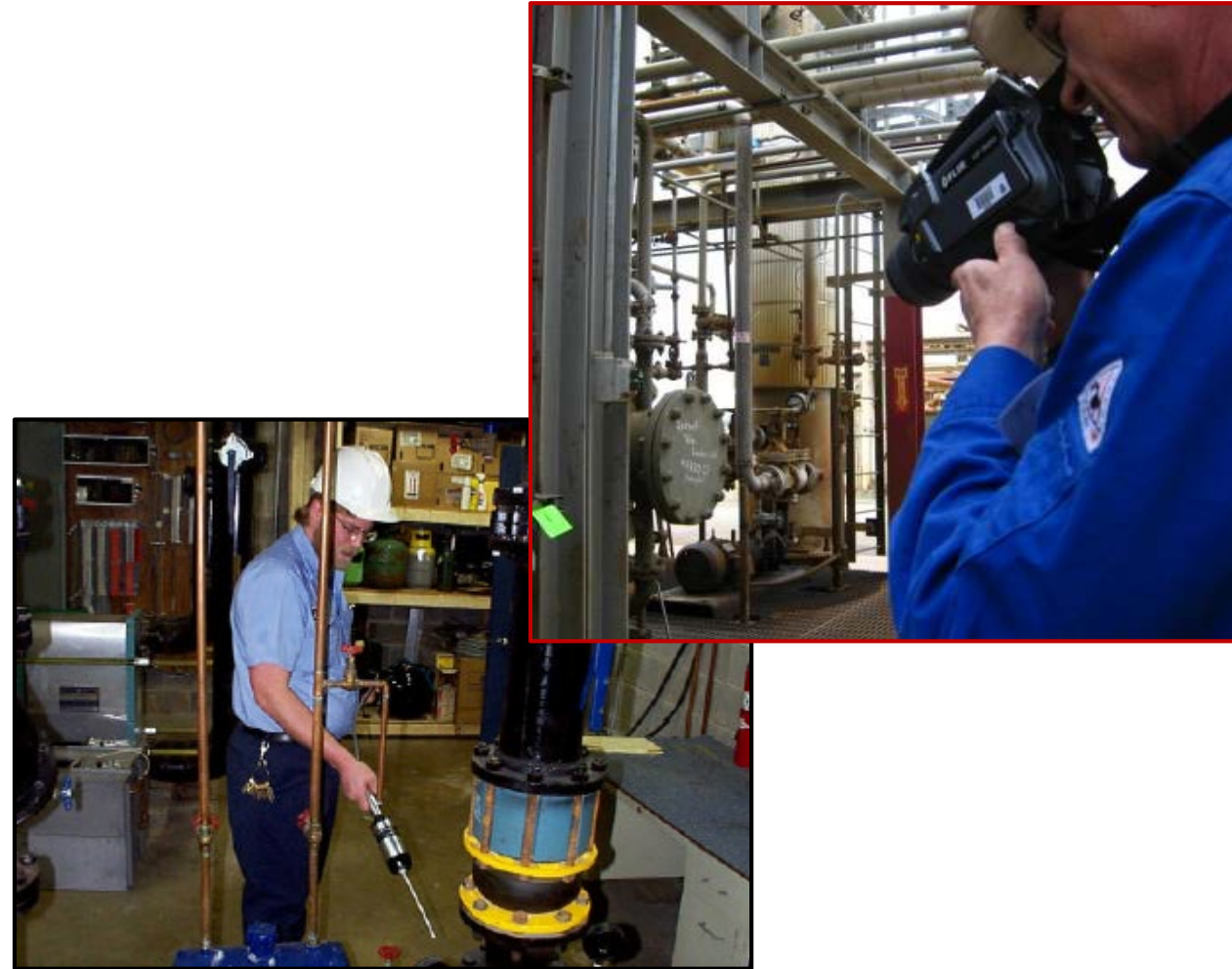
Inspecting pipes for leaks using an OGI camera (top); Manual leak detection (EPA Method 21) using a VOC detector probe (bottom)
