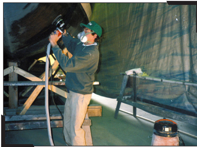
To minimize the spread of the debris, dust and paint chips, try to do all work in a covered building (Source: Jay Tanski, New York Sea Grant).
