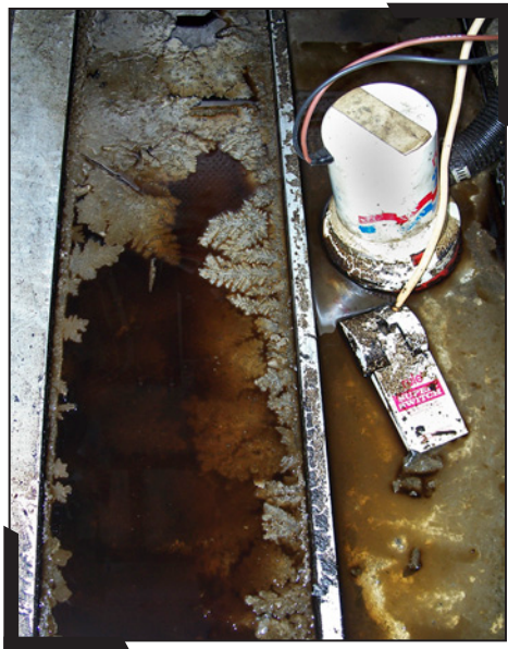
The use of a bilge sock would help prevent oil collected in the bottom of this bilge from being discharged to the lake (Photo by Joe Exl, IDNR).
