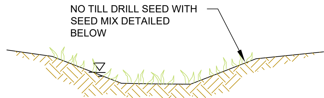
GRASSED WATERWAY - TYPICAL SECTION NOT TO SCALE
