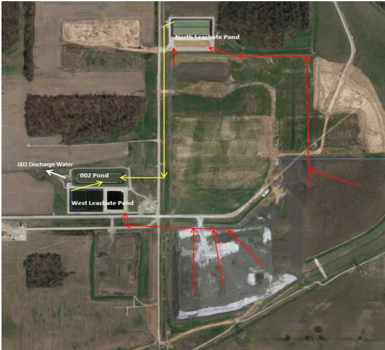
Figure 4: Outfall 002 Pond System
