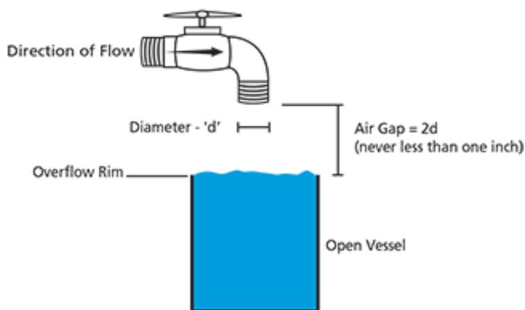
Although an air gap generally affords maximum protection, it can be bypassed easily, its effectiveness thus being entirely destroyed. It is also not reliable if the gap is too small. As defined in USC and Indiana Plumbing Code, *an air gap should be twice the diameter of the effective opening of the supply pipe. In no case shall the gap be less than one inch, or 25.4 mm.*
