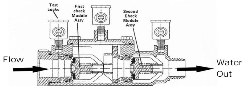
This device is one of the oldest types of backflow preventers, dating back to the late 19<sup>th</sup> century. The DCV protects against non-health hazards only under backpressure and backsiphonage conditions. An approved double-check valve assembly is regarded as an assembly that meets the requirements of USC, CSA or ASSE.
