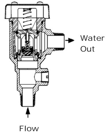
**Pressure Vacuum Breaker and Spill Resistant Vacuum Breaker**
