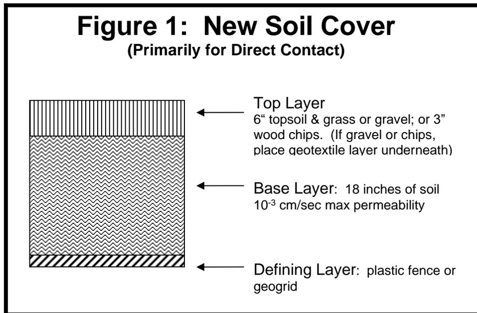
The top layer should be made of topsoil with grass covering the surface. The purpose of the top layer is to armor the cover surface to prevent significant erosion or structural deterioration. Selection of materials may be based on site usage.
