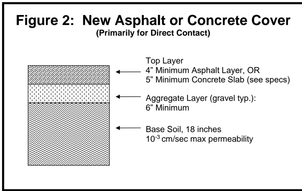
The asphalt top layer should contain two lifts of asphalt with a minimum thickness of 2" per layer.
