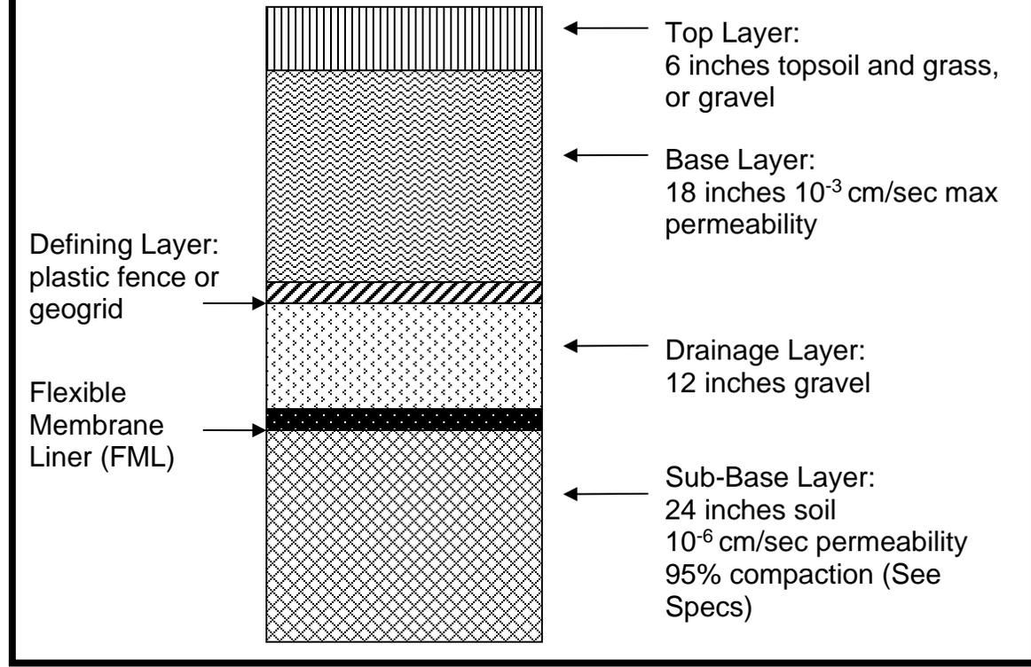
The direct contact layers are identical to the direct contact design, except as noted where a fabric filter should be used as the defining layer to prevent base layer soil mixing and clogging of the drainage layer.
