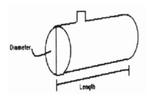
The capacity of a liquid tank spreader is the easiest to calculate. The capacity is often painted on the side of the tank. If capacity information is not available, use the following steps to calculate the capacity (in gallons) of your spreader.
