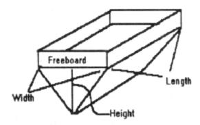
V-bottom spreaders can hold either semi-solid (gallons) or solid manure (tons). If you do not have the capacity of your spreader, you will have to make three measurements.
