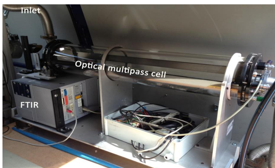
Figure A 3. The MeFTIR instrumentation consisting of a Bruker FTIR spectrometer connected to an optical multi-pass cell.
