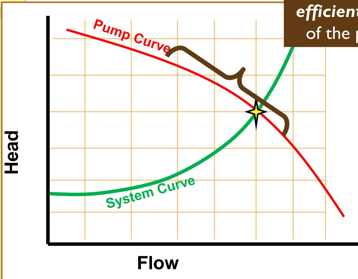
The point of intersection of the two curves is where the pump will operate in the system.
