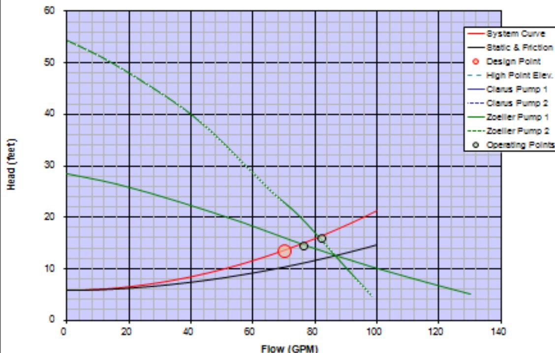
NOTE: THE DISPLAYED PUMP CURVES HAVE BEEN ADJUSTED TO ACCOUNT FOR THE EFFECT OF THE WEEP HOLE
