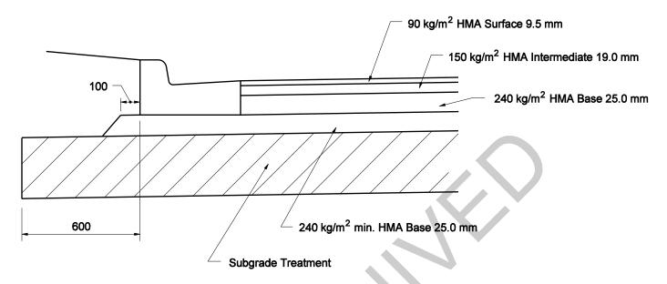
Note: See Section 52-9.02 to determine the appropriate HMA mixture designation.
