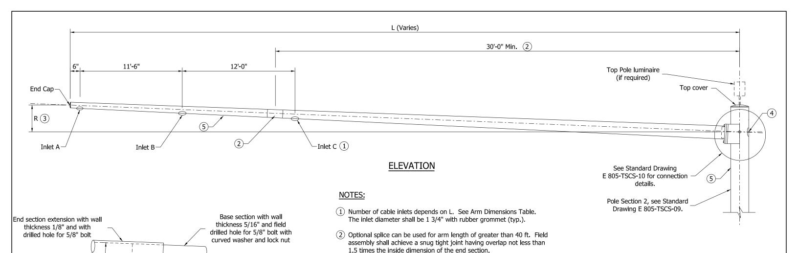
(3) Arm rise R is measured in the undeflected position without vertical
