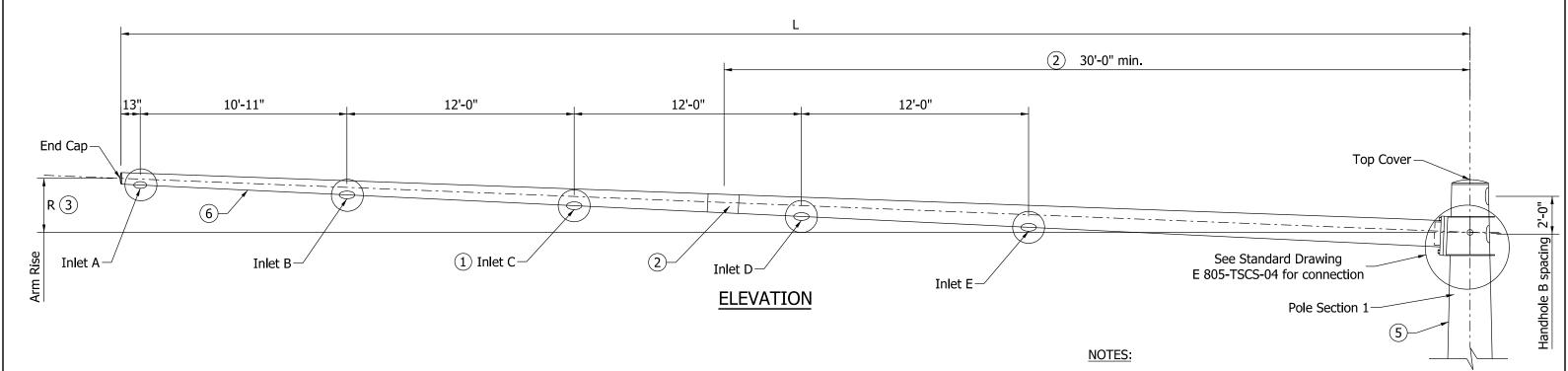
End section extension with wall thickness 3/16" min. and with drilled hole for 5/8" bolt 2R End sect. 5/8" thru bolt ≥3R
