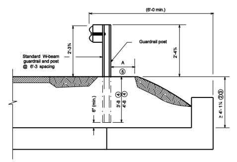
GUARDRAIL ASSEMBLY FOR COVER ≥ 4'-11/4
