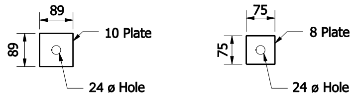
BACKING PLATE Skewed Structure Only
