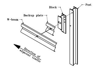
W-BEAM SPLICE CONNECTION DETAIL AT POST FOR NON-SPLICE CONNECTIONS All dimensions are in mm unless otherwise specified.
