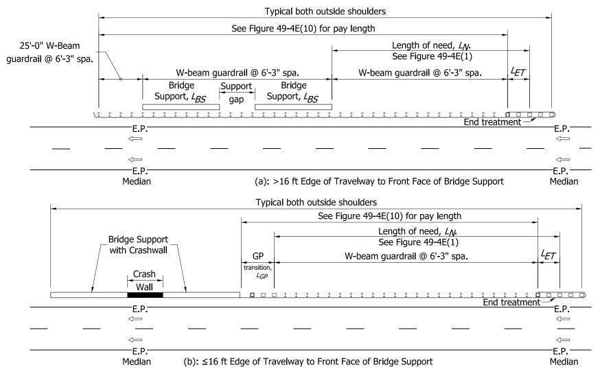
GUARDRAIL CONFIGURATION FOR BRIDGE SUPPORT INSIDE CLEAR ZONE, ONE-WAY ROADWAY, TWIN OVERHEAD STRUCTURES, OUTSIDE SHOULDER
