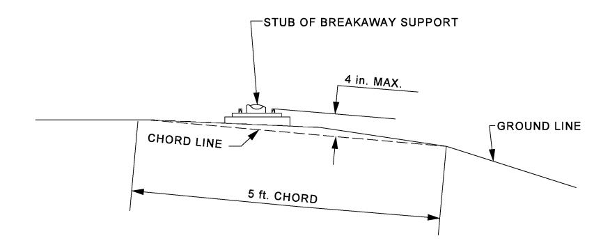
BREAKAWAY SUPPORT STUB CLEARANCE DIAGRAM
