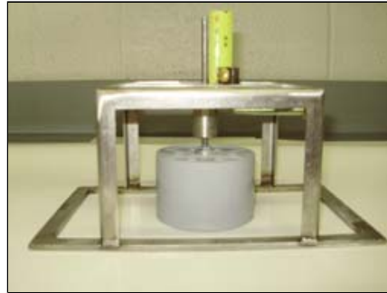
Apparatus used in ASTM C1712. Photos: BASF
