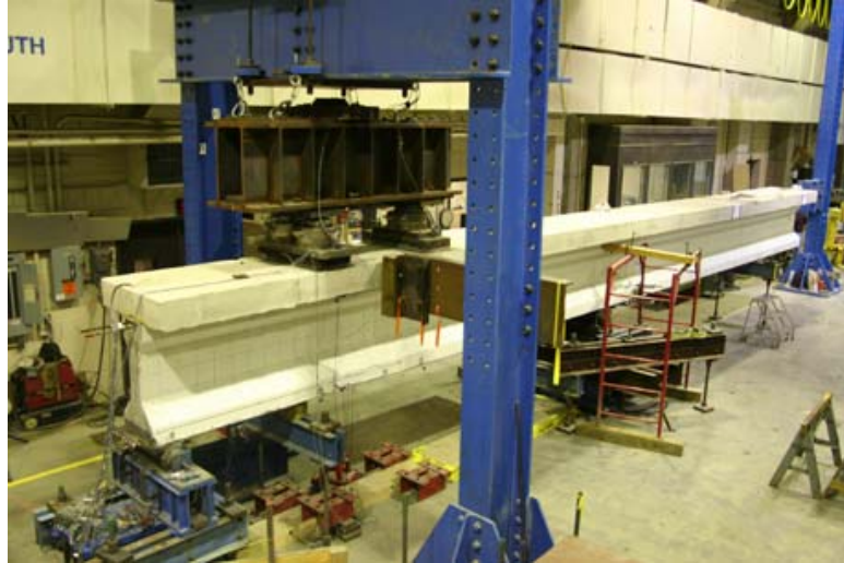
Strand development length test of LWHPC beam.
