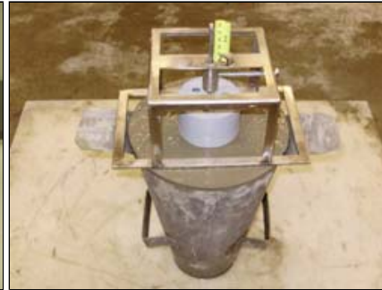
Apparatus used in ASTM C1712. Photos: BASF
