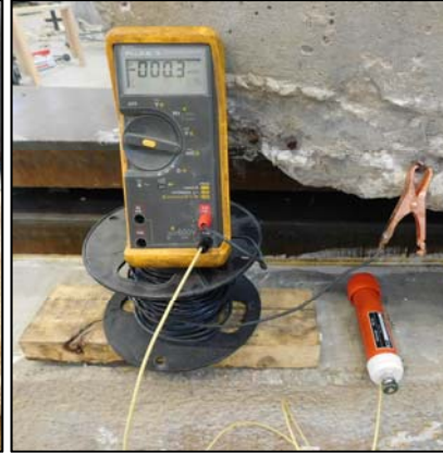
Half-cell potential measurement
