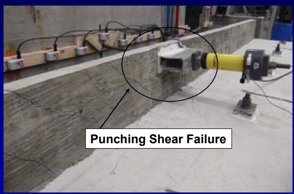
Specimen #1L at 29.2 kips
