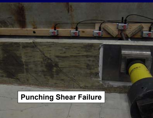
Specimen #2L at 23.7 kips
