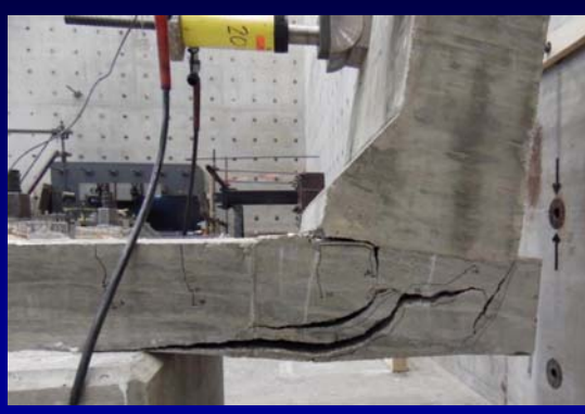
Typical Specimen Failure Plane
