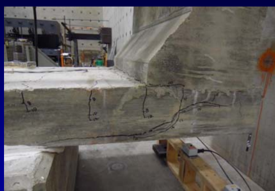
#5 Epoxy @ 3.5" Hooked 15 kips
