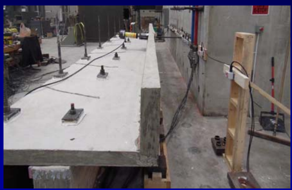
Specimen #1L at 29.2 kips
