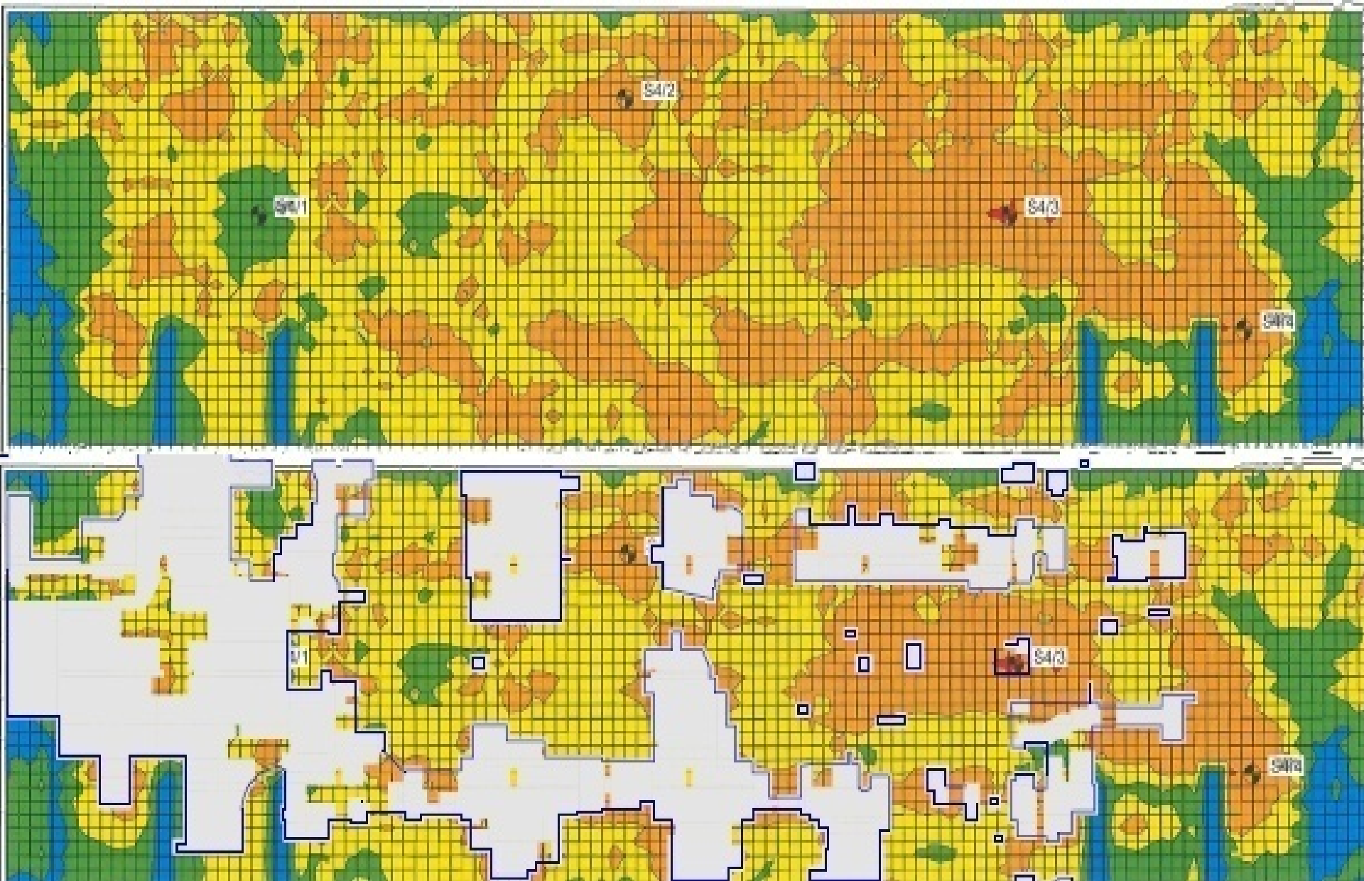
Corrosion Potential Mapping Overlaid with Delamination Survey
