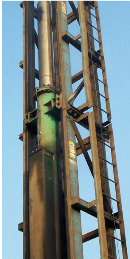
Figure 12. Piston Extending from the Top of the Hammer. (Note ring on the piston)
