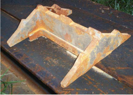
Figure 9 Tip (Bottom) of Pile Shoe
