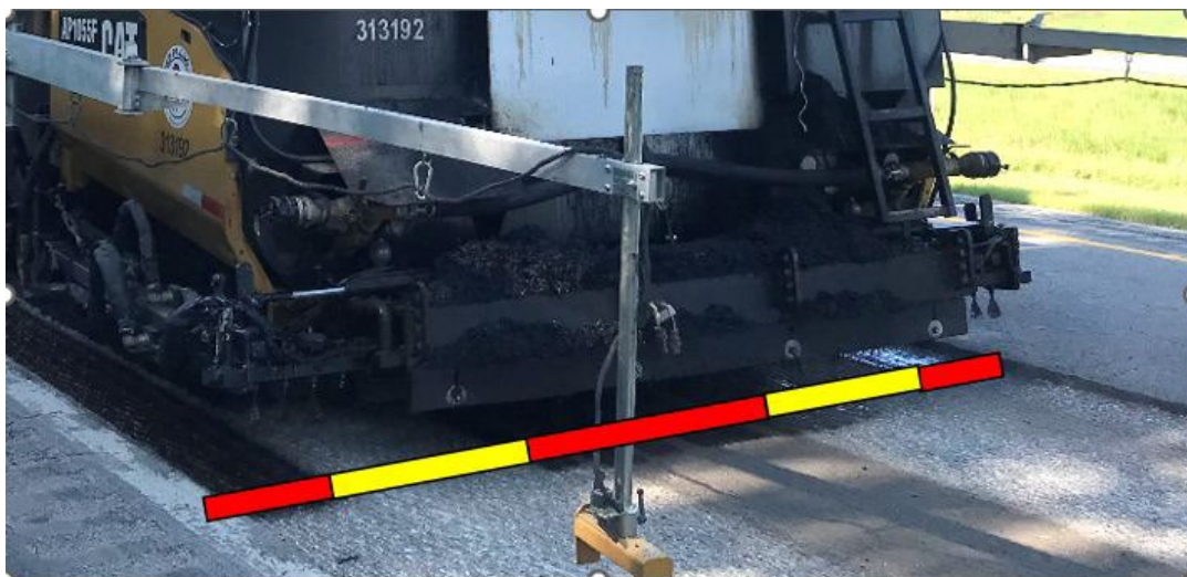
Figure 13.24-3d. Spray Paver Emulsion Application Locations Red indicates front nozzle application, and Yellow indicates rear nozzle application
