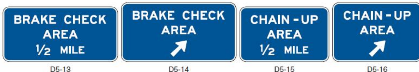
Figure 2I-6. Brake Check Area and Chain-Up Area Signs
