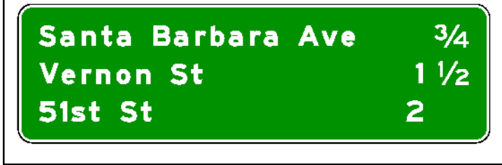
Figure 2E-31. Interchange Sequence Sign
