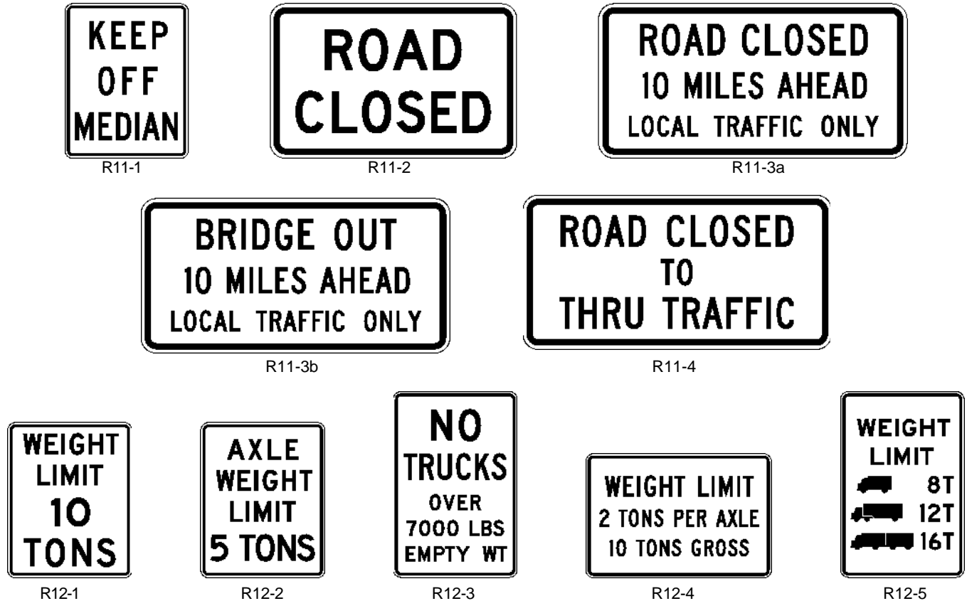
Figure 2B-29. Road Closed and Weight Limit Signs
