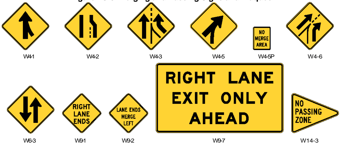
Figure 2C-8. Merging and Passing Signs and Plaques
