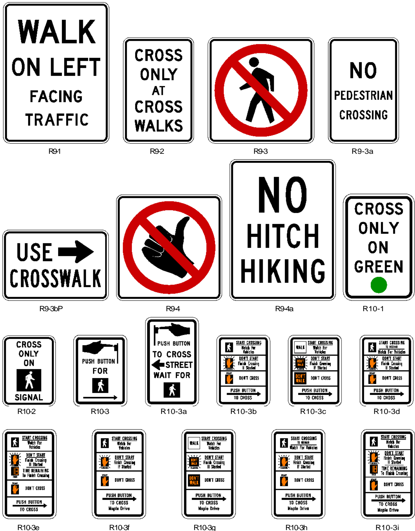
Figure 2B-26. Pedestrian Signs and Plaques (Sheet 1 of 2)
