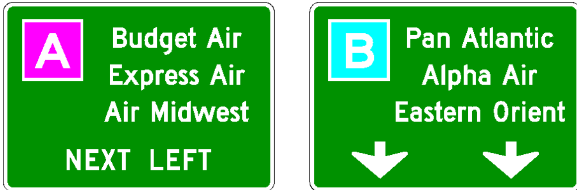
Figure 2D-1. Examples of Color-Coded Destination Guide Signs
