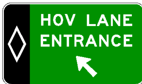
Figure 2G-6. Examples of Overhead or Post-Mounted Preferential Lane Entrance Direction Signs
