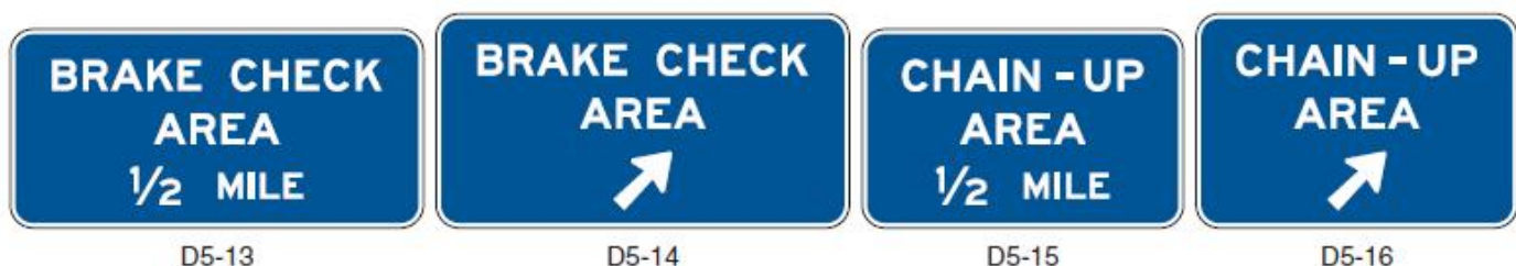
Figure 2I-6. Brake Check Area and Chain-Up Area Signs
