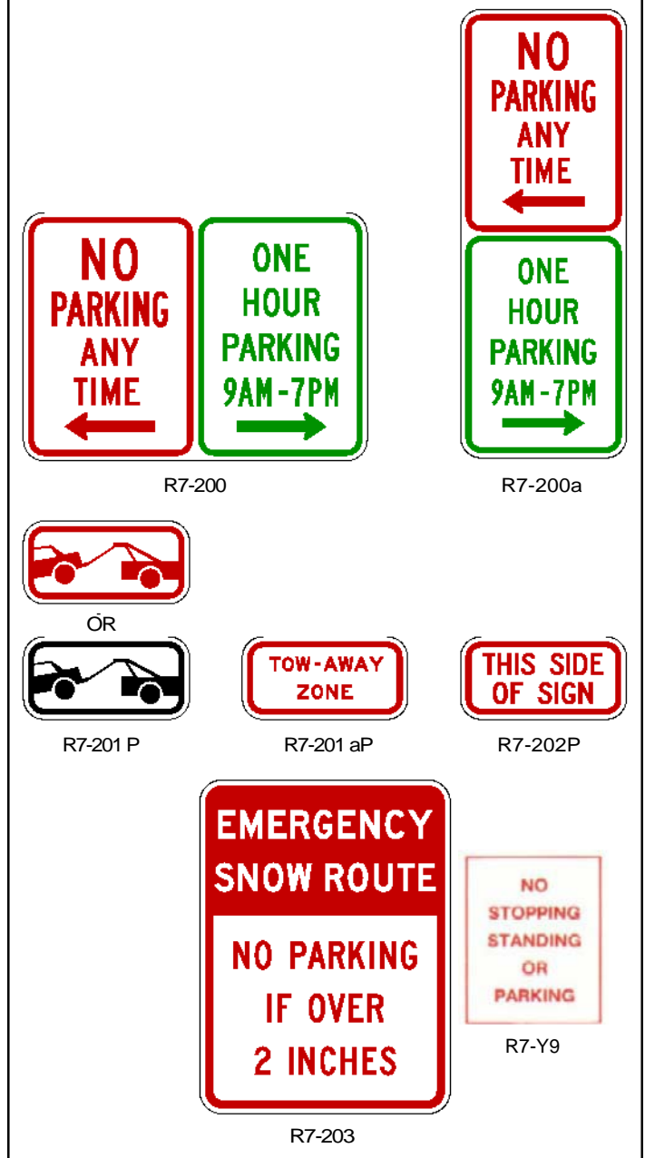
Figure 2B-24. Parking and Standing Signs and Plaques (R7 Series) (Sheet 2 of 2)
