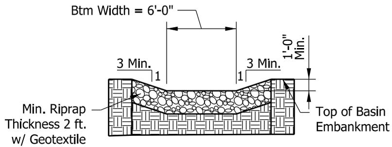
**CROSS SECTION AT EMERGENCY SPILLWAY SECTION C-C**
