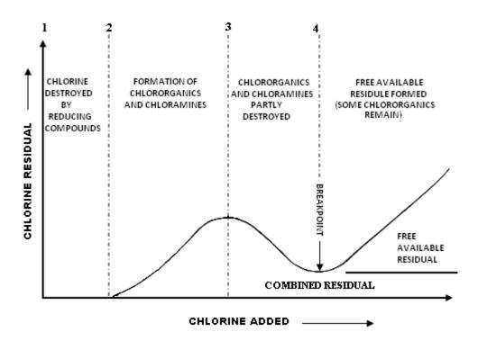
Between points 2 and 3, the chlorine reacts with organics and ammonia naturally found in the water. Some combined chlorine residual is formed – chloramines.
