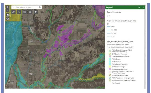
This screenshot of a portion of Otter Creek and the Wabash River in Vigo County shows the FEMA Special Flood Hazard Area (SFHA) from the Flood Insurance Rate Maps in the blue and red hash and the additional stretches of stream that have been modeled by the Division of Water in purple and yellow/black.
