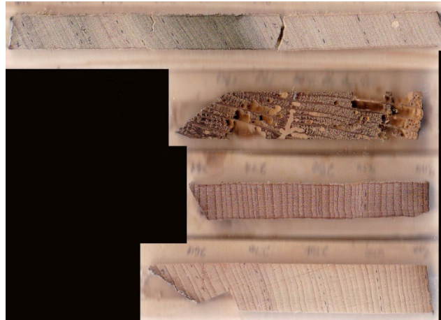
Figure 5. Sanded and mounted cores from the Bronnenberg I-house. From top to bottom: tulip poplar BIH13B; white oak BIH24A; beech BIH02A; and white pine BIH07A. The outermost ring in each sample is to the right. Note the variation in ring width; this variation is necessary for accurate crossdating (Photo credit: Darrin L. Rubino).
