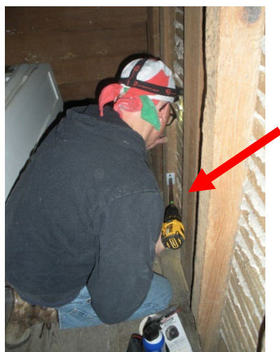
Figure 4. Collecting a core sample from a closet under the main stairway at the Bronnenberg I- House. The arrow points to the borer chucked in a drill (Photo credit: Christopher Baas).
