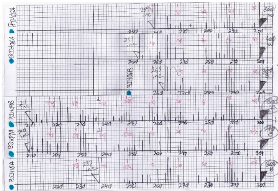
Figure 6. Skeleton plots created for six beech samples obtained from the Bronnenberg I-house (Madison County, Indiana). In the plots, each line of the strip of graph paper represents one year. A vertical line is drawn to represent the inverse size of a ring (the larger the line, the smaller the tree ring) so as to highlight decreases in annual growth when neighboring rings are compared. The plots are slid along each other to match the pattern and size of lines made for various years. The values in red represent decades that were determined via crossdating (Photo credit: Darrin L. Rubino).
