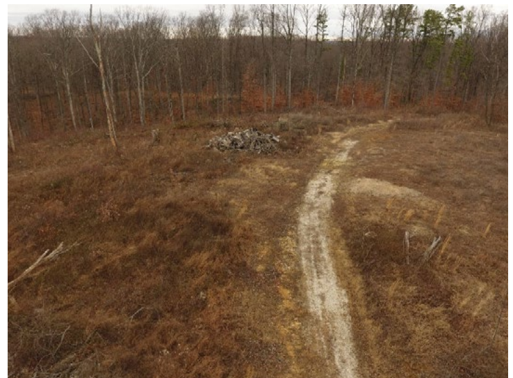
Access road is the lane that connects log landings to municipal roads. Here an access lane approaches a log landing. Drone photo taken on state forest property by Jamie Winner, DNR.
