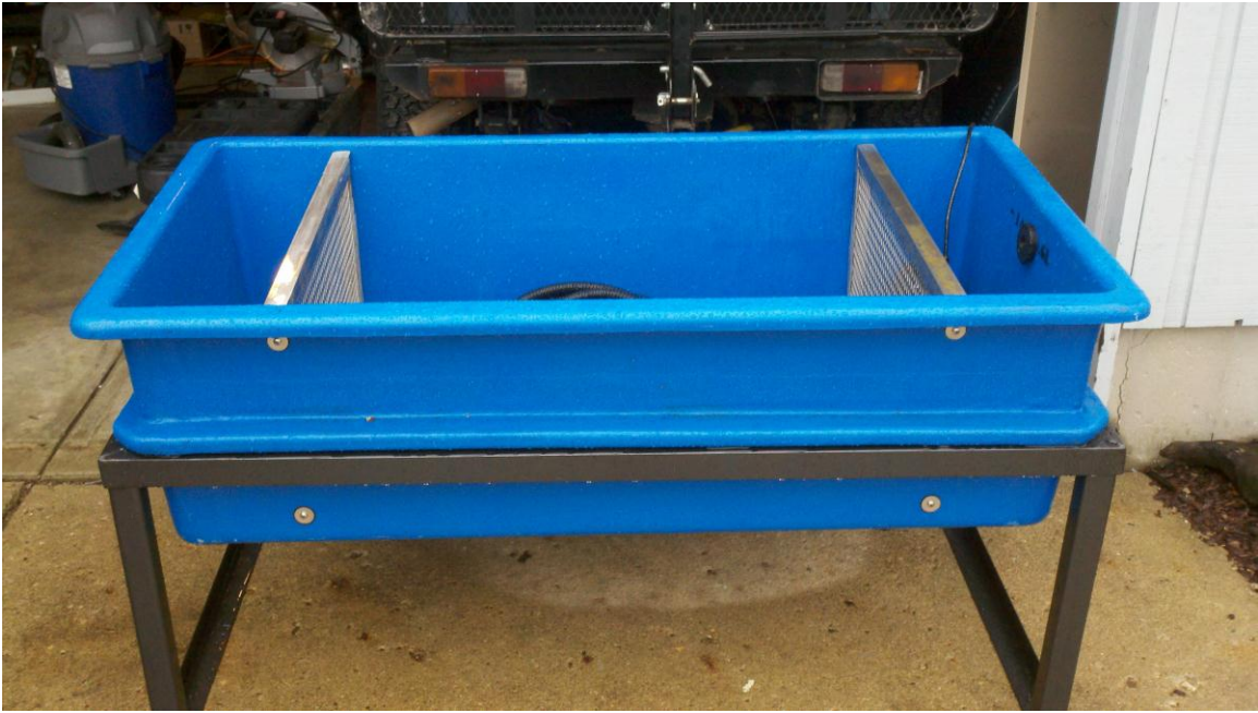
Plate 1. Mobile electroanesthesia unit (MEU) tank with stainless steel electrodes and stand installed.
