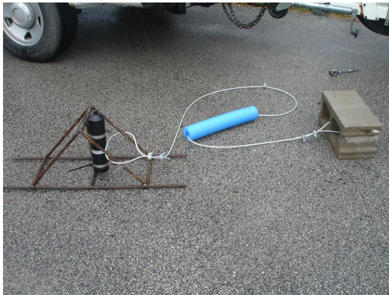
Plate 6. Smaller deployment system used for Vemco VR2W passive receivers in shallow reaches of the Wabash and Little Rivers.
