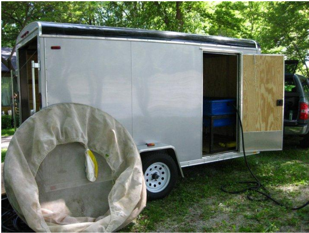
Plate 3. Mobile electroanesthesia unit (MEU) with flow through system of pumped river water in operation.
