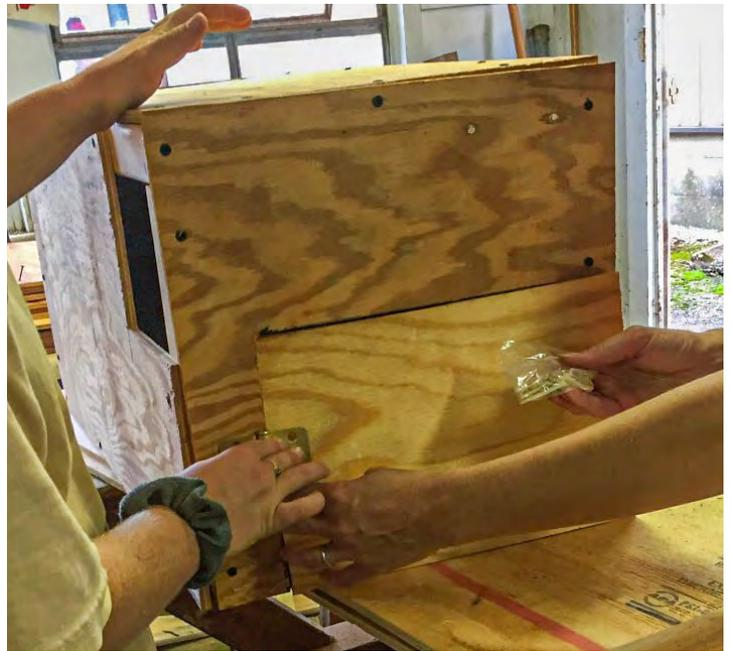
NOTE: If the end of the screws for the hinge protrude into the box, please take a piece of scrap plywood and place it behind the door. Then attach the hinge into place so the screw goes through the door and into the scrap wood. This will prevent the screws from injuring birds in the nest box.
