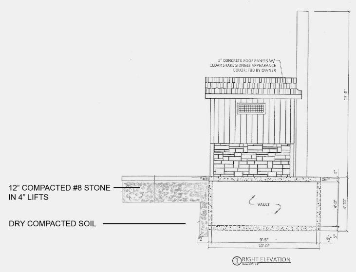
OVERDIG OF VAULT IN THE FRONT OF THE UNIT IS TO BE BACKFILLED WITH COMPACTED #8 STONE
