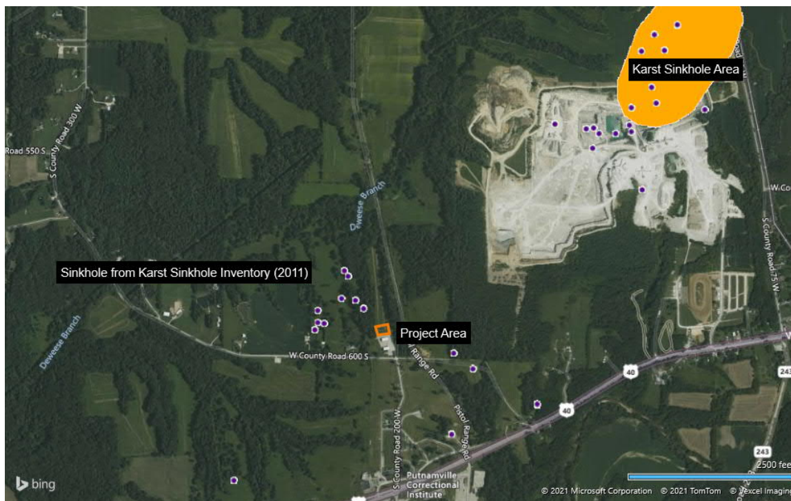
Figure 1. Mapped karstic features near the project area per Indiana Map GIS System
