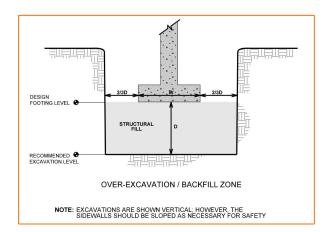
Consideration could also be given to the use of lean concrete in undercut areas extending to bear directly on deeper suitable soils as illustrated on the sketch below. We recommend a contingency be included in the contract to account for undercutting and fill placement and compaction as needed to address poor foundation subgrade conditions.
