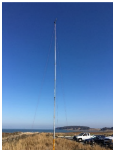
Figure A 5. The FluxSense mobile wind mast with an RM Young anemometer mounted on top. The mast could be erected from 3 to 10 m.
