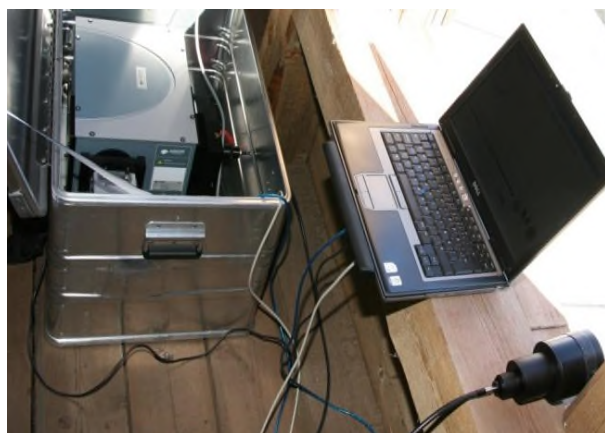
Figure A 2. The mobile SkyDOAS system: Telescope, optical fibre, spectrometer and control computer.
