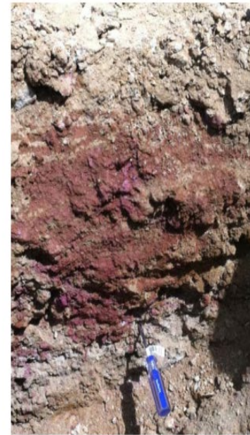
(a) Well mixed lime-soil modified soil
