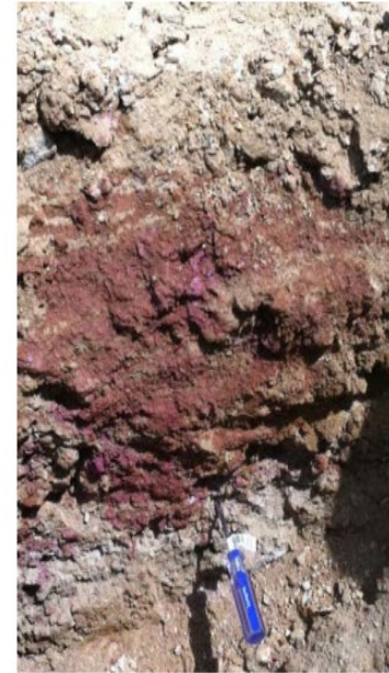
(a) Well mixed lime-soil modified soil
