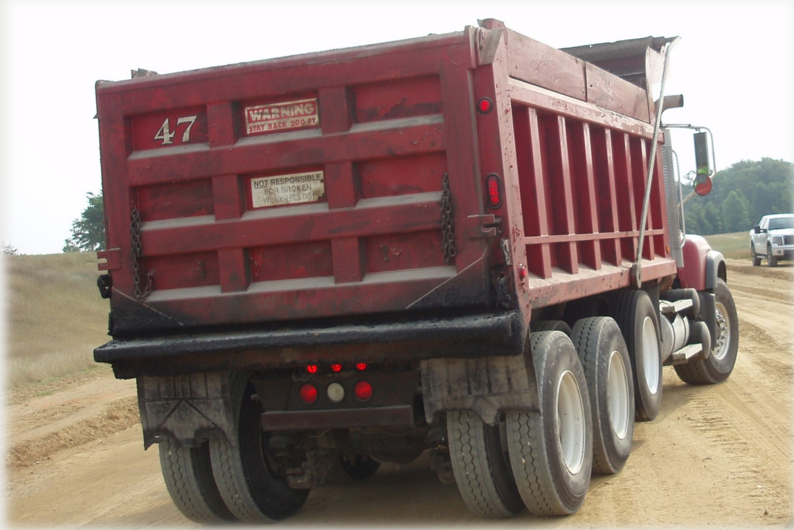
A fully legally loaded tri-axle dump truck. ( About 35 t.)
