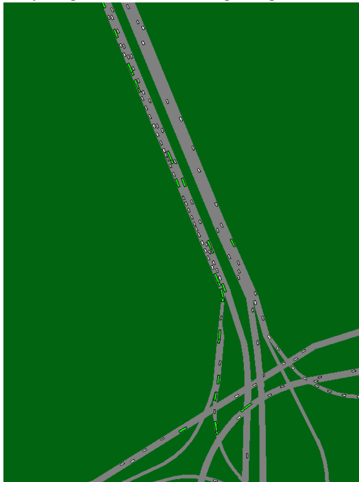
Figure 6 – I-65 SB Kennedy Bridge Bottleneck and Queuing During AM Peak Hour
