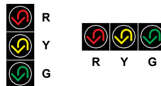
Figure 4E-1. Typical Arrangements of U-Turn Signal Faces
