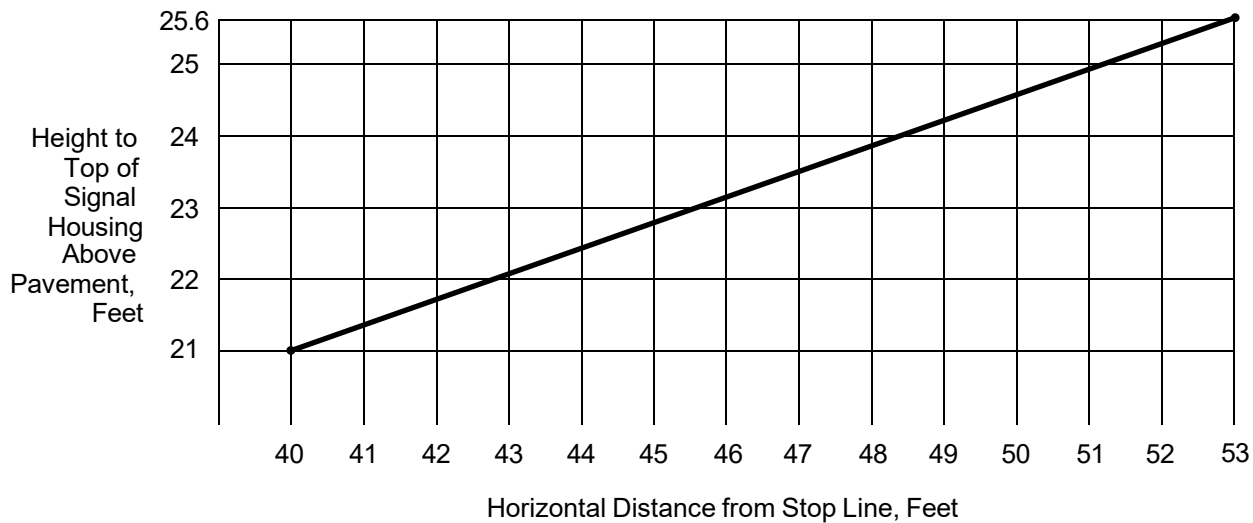
Figure 4D-3. Maximum Mounting Height of Signal Faces that Are Located between 40 Feet and 53 Feet from the Stop Line
