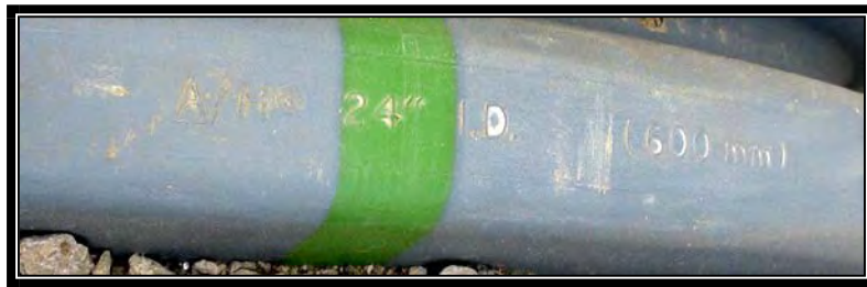
Figure 12-1: Raised Markings on 24 in. Polypropylene Pipe
