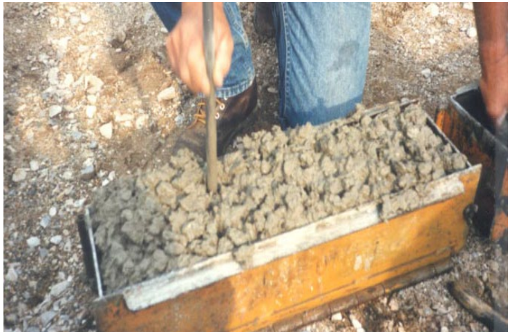
Figure 3-3 Concrete Beam Used for Flexural Testing
